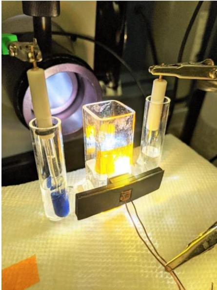
*The team's experimental water-splitting apparatus.*
